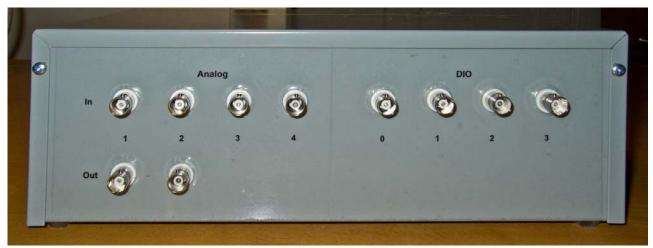
The rear panel includes input and output triggers for analog acquisition and playback and control signals for two timer channels:
